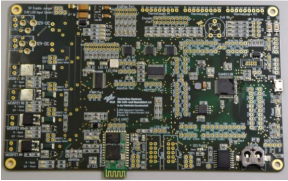
Figure 16: Custom PCB used for Concept B control and data acquisition
