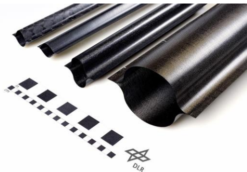
Figure 1: Rollable DLR-Booms in various cross section versions
