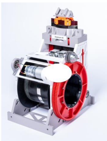
Figure 9: Boom deployment mechanism demonstrating Concept A
