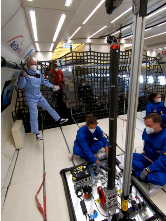
Figure 19: Concept A fully deployed (during parabola #20).
