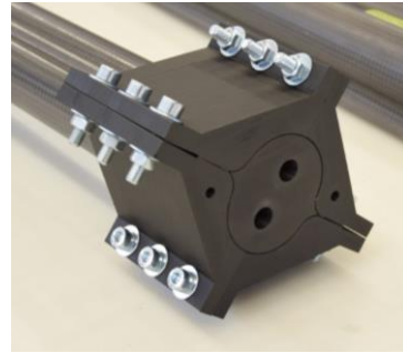
Figure 4: Ideal, solid boom interface for laboratory stiffness testing
