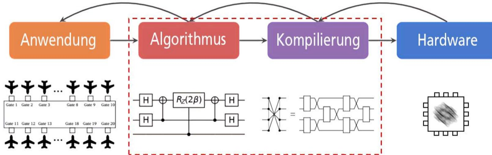
*Hardware-Software Co-Design: Efficient compilation of quantum circuits and customised quantum algorithms for industrial application problems (Source: DLR).*
