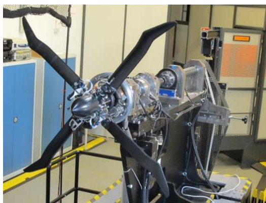
Figure 1: Rotor Test Facility Göttingen with four-bladed rotor
