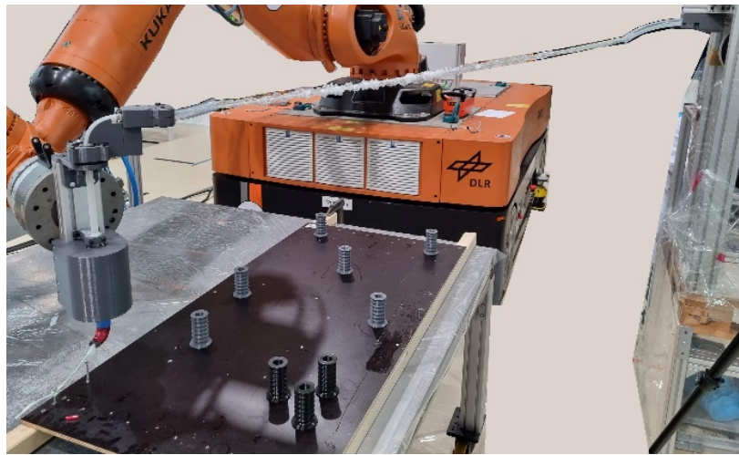
Figure 2: Robotic processing of reinforcement strands produced by the DWM
