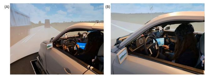
Fig. 2. Driving simulator with participant. Left. The manual driving mode; Right: the automated driving mode with interaction with the user interface.
