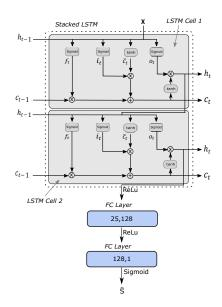
Fig. 12. LSTM layer structure adapted from [58]
