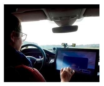
Fig. 8. Setup in the automated vehicle: the driver was interacting with a user interface while the car was driving fully automated in Study 2.
