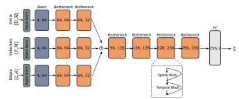
Fig. 10. Layer structure of one of the channels of the Fast&Slow network adapted from [51]
