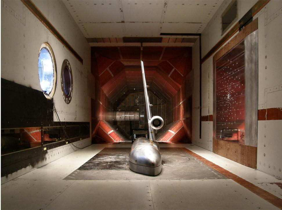
Figure 3.3: Photo of Do728 model and microphone array in the closed wind tunnel test section.
