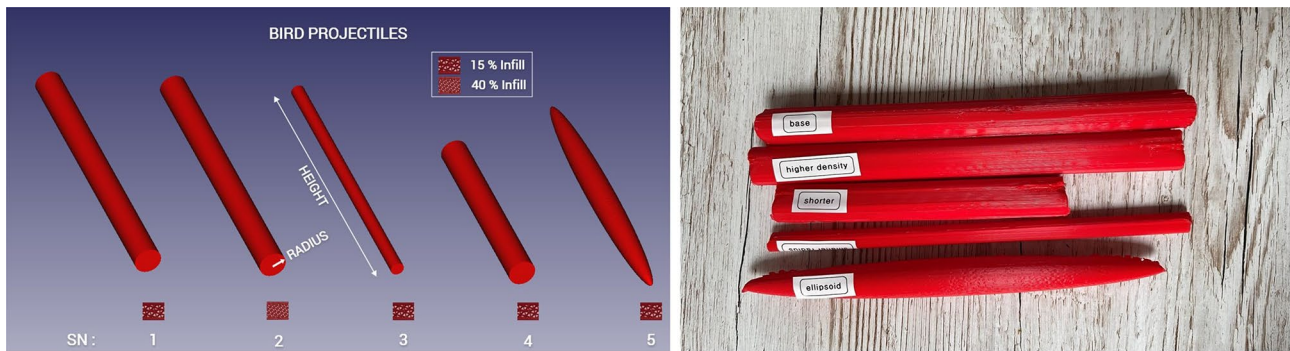
Fig. 2 CAD models and 3D prints of the bird projectiles
