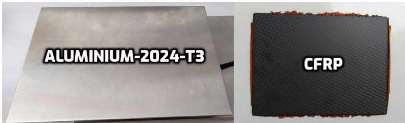
Fig. 3 Test specimen for the bird strike experiment. Left: Aluminium-2024-T3; right: CFRP
