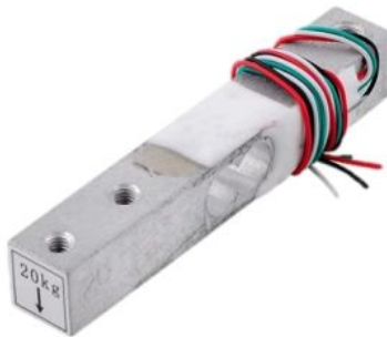
Fig. 4: Procured load cell force sensor
