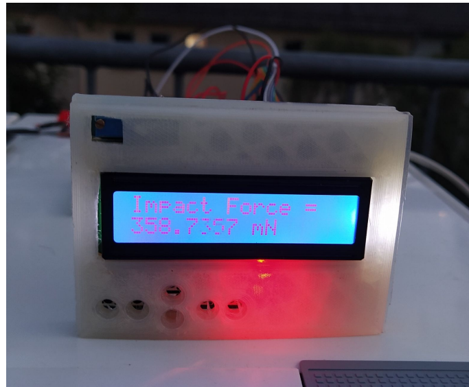
Fig. 6: 16x2 Liquid Crystal Display unit
