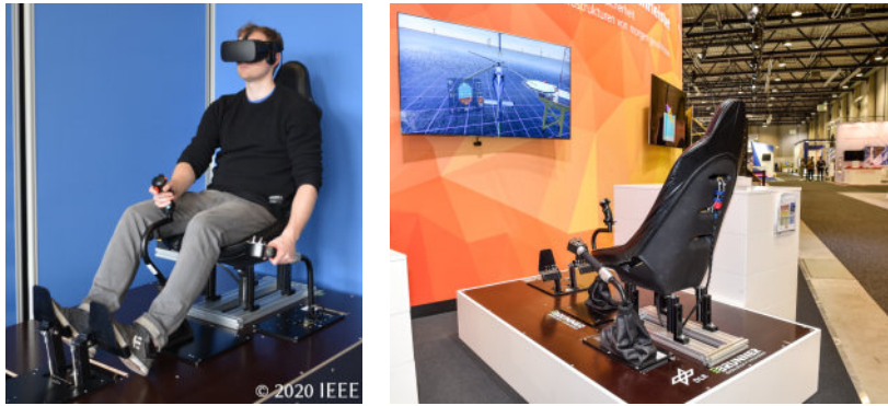
(a) Pure VR setup with goggles and controls only [70, 72]. (b) Exhibition setup with additional external monitor for spectators (here at ILA Berlin 2018).
