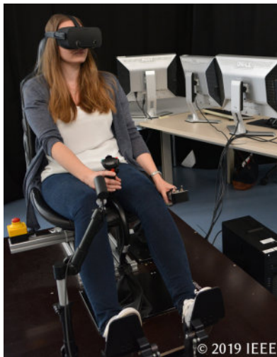
(a) Study I – Fully virtual setup with a pilot wearing the Oculus Rift VR goggles.
