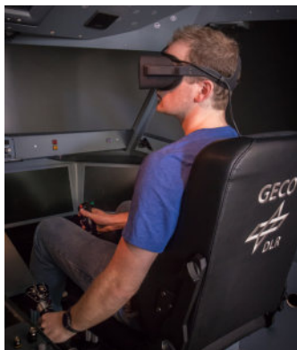
Figure 7.8 – Experimental setup with a pilot wearing the Oculus Rift CV 1 VR-HMD in DLR's GECO simulator.
