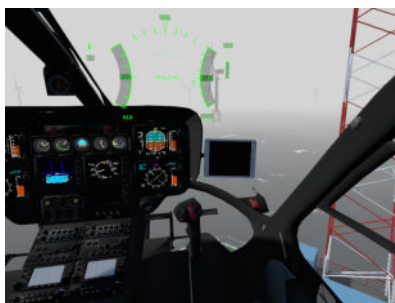
(b) Partially virtual cockpit with optical see-through HMD — A head-up PFD symbology augments the pilot's natural view.
