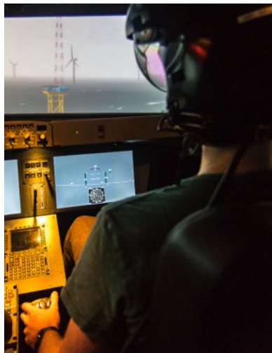
(b) Study II – Pilot wearing the JedEye see-through HMD in the GECO simulator.
