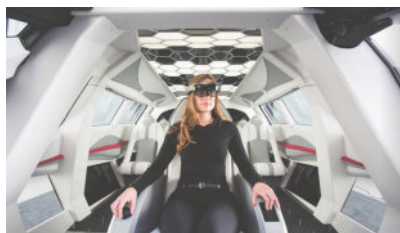
(a) Mockup of Bell's FCX-001 cockpit using an optical see-through HMD as the only display [o].
