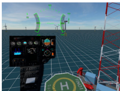
(c) Partially virtual cockpit with video see-through HMD — A video stream of the conventional display panel is integrated into an otherwise virtual view.
