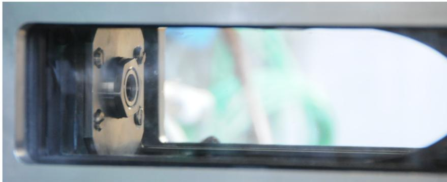
Figure 4: Photo of injector element integrated into the M3.1 micro-combustor.
