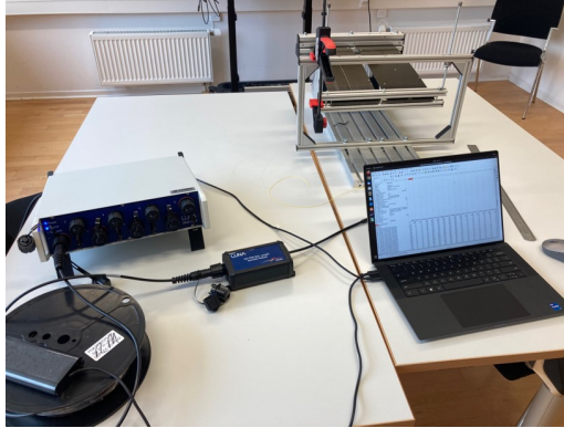
Figure 8: FOSS system during the measurement. Test stand in background
