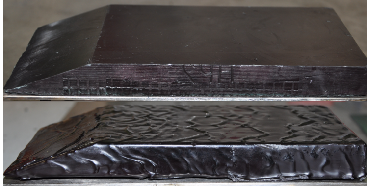
Fig. 2 Fuel slab configuration with initial slope on the left-hand side before (top) and after (bottom) combustion test, adapted from Rüttgers et al. [6].
