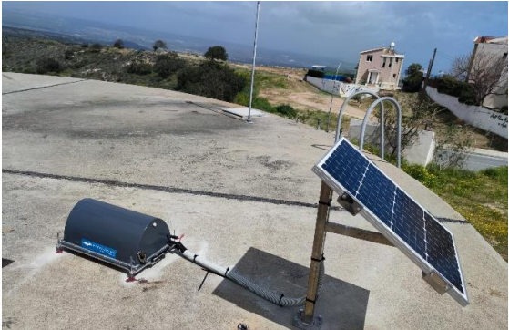
Use of Electronic Corner Reflectors for the first time in Cyprus
