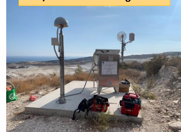
Example of a Mobile GPS/GNSS CORS Configuration
