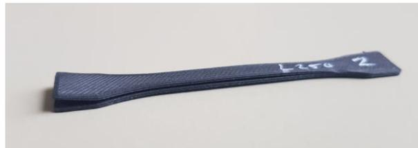
Figure 8: Specimen printed at 250 °C air temperature.
