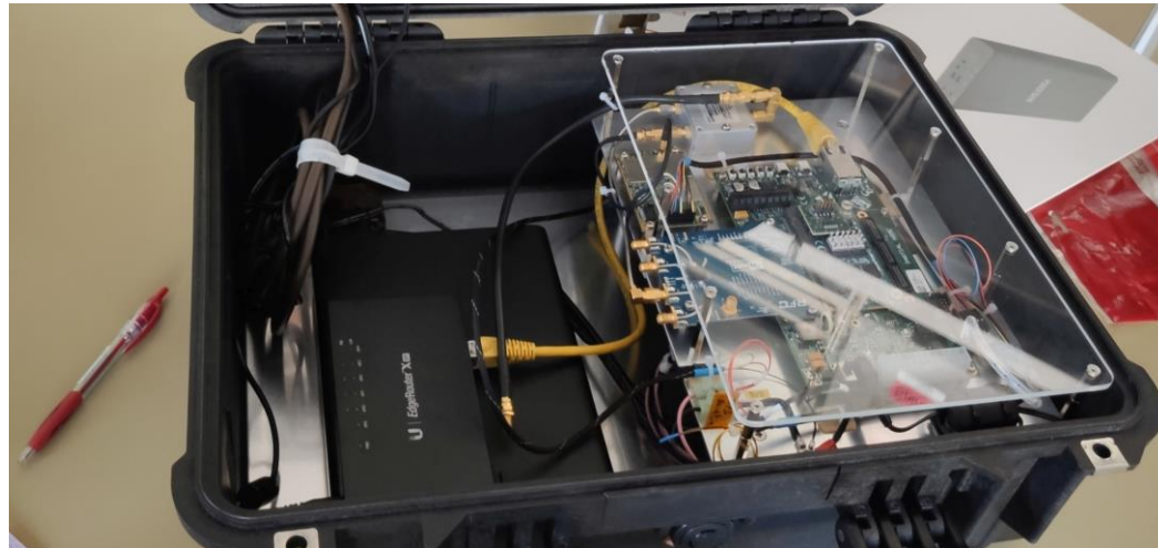
Photo: PACO Receiver unit for ground-based testing
