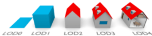
Figure 3: The five different LoDs for building models in CityGML (Biljecki et al., 2016). Licensed under CC BY-NC-ND 4.0.
