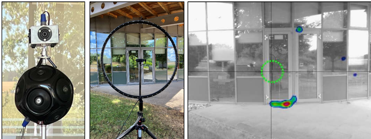
Figure 2: Measurement setup: pair of loudspeakers inside (left), microphone array or acoustic camera outside (centre), visualization of the loudest noise sources on the facade (right).
