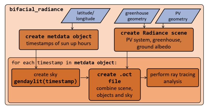
workflow of the model implemented in bifacial\_radiance based on Radiance [5,6] validation with data from literature
