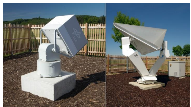
Figure 1: “Kalibri” transponder and 2.8 m corner reflector.
