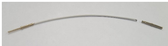
Fig. 9. Wire with low cycle fatigue failure.
