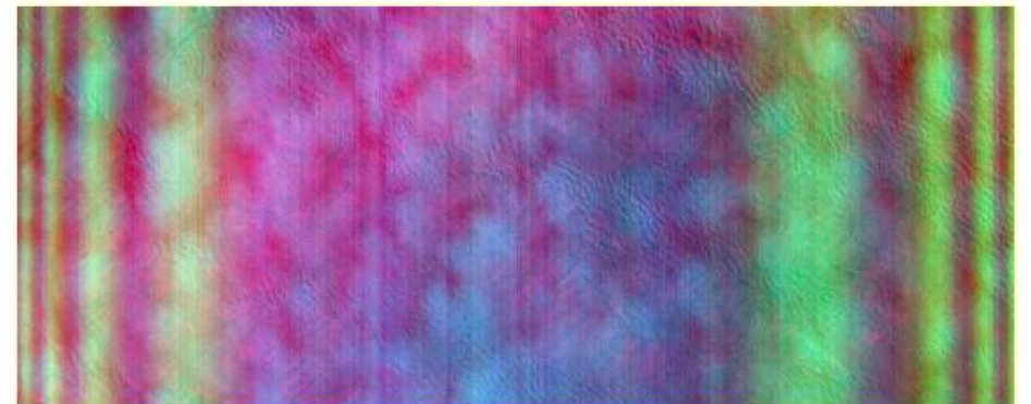
Figure 6-23 Fringing of the VNIR, Principal Component-transformed data
