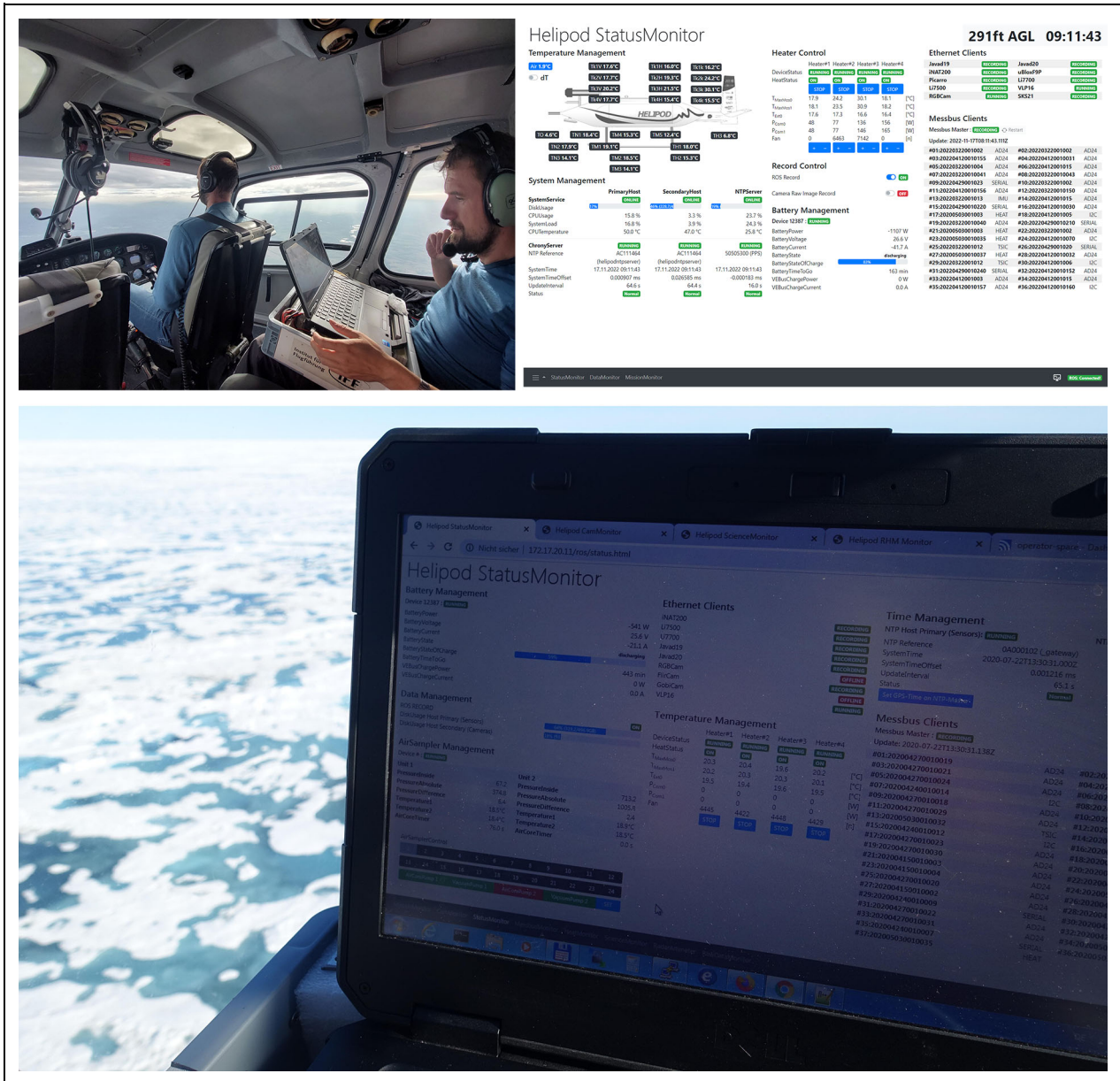
Figure 8. Remote WiFi access to the HELiPOD during flight. A specially developed user interface enables to monitor the current state of the whole system and sensors. Life sensor data are displayed allowing operational decision-making. A control of sensors and temperature management is given.
