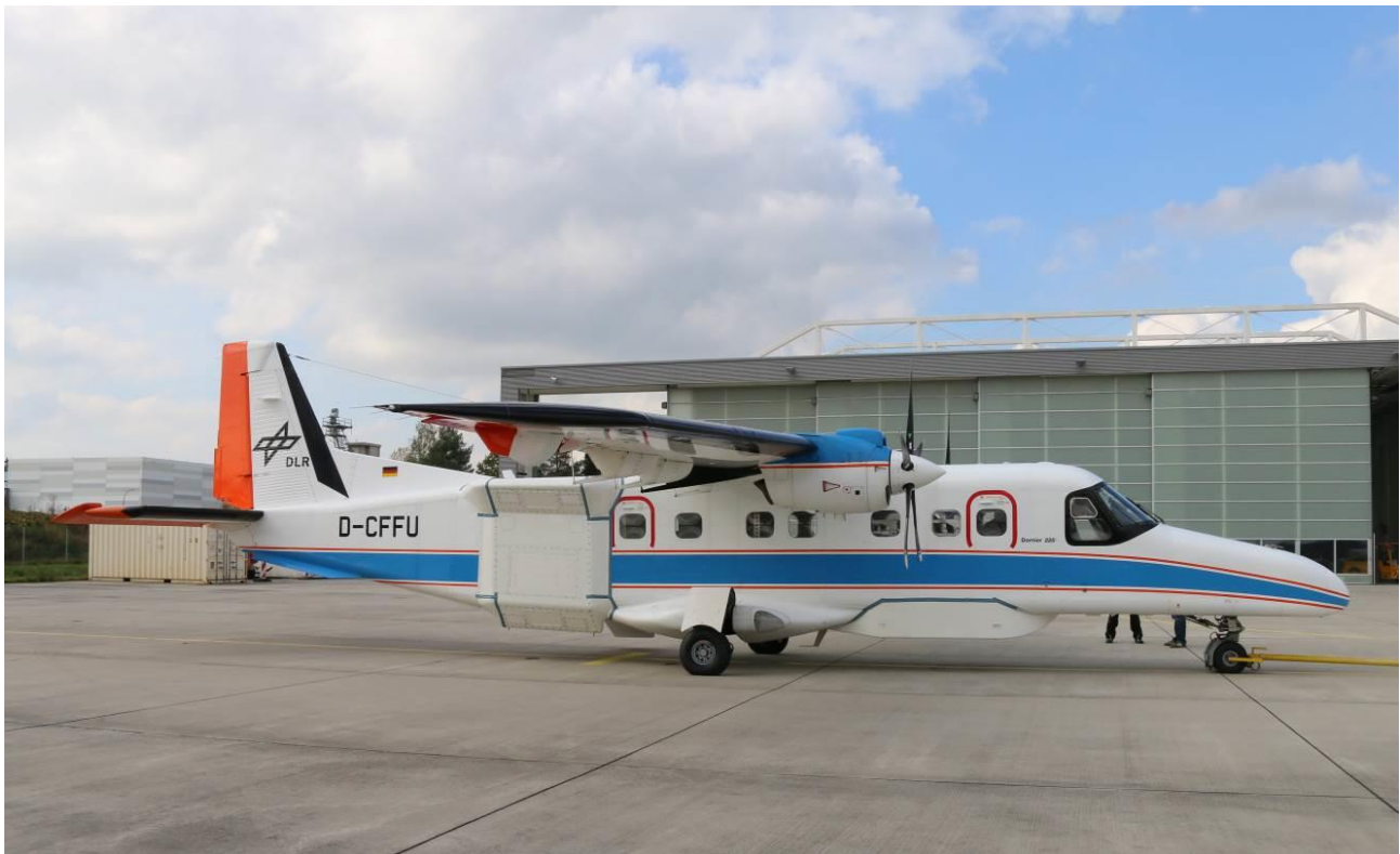
Figure 2-1: The F-SAR instrument on-board a DLR Dornier DO 228 aircraft. Antennas are mounted behind the wing (X-C-S-L) and under the cockpit (P).
