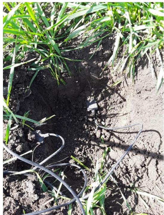
Figure 3-6: Example of temporary station set-up, equipped with soil moisture and temperature sensors at 5cm and 20cm and dielectric leaf wetness sensor.
