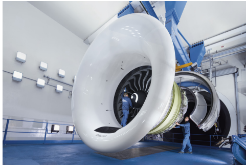
FIGURE 2: BELLMOUTH AIR METER.
