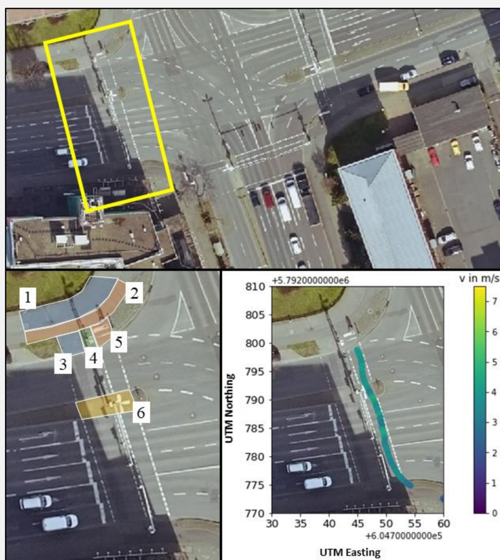
Figure 2. AIM Research Intersection in Brunswick, Germany; orientated North. Top: Satellite image of AIM Research Intersection (yellow: area of interest for this analysis). Bottom, left: Detailed view of the area of interest with polygons (1: footpath, 2: bicycle path, 3: waiting area and stop line for pedestrians, 4: space between pedestrian and bicycle waiting areas and stop lines, 5: waiting area and stop line for cyclists, 6: crossing aid). Bottom, right: An example trajectory of a cyclist on the bicycle path in map projection system UTM 32U. Orthophoto source: DLR e. V.
