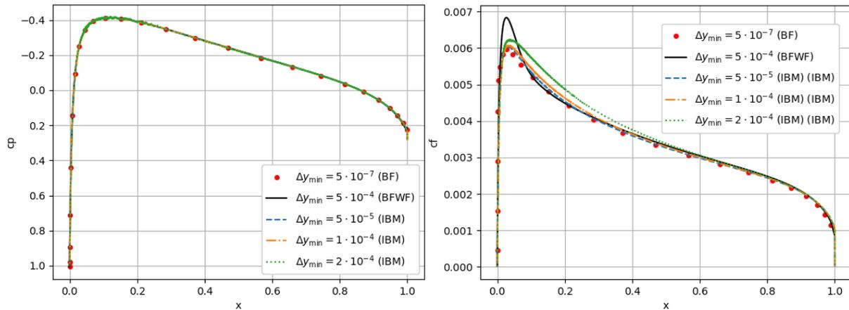
**Figure 2.** Pressure and friction distribution of NACA 0012,  $M=0.15$ ,  $Re=6E6$ ,  $AOA=0^\circ$  for body-fitted (BF: circles), body-fitted with wall function (BFWF: solid), and IBM with three sizes (dashed, dashdot, and dotted).
