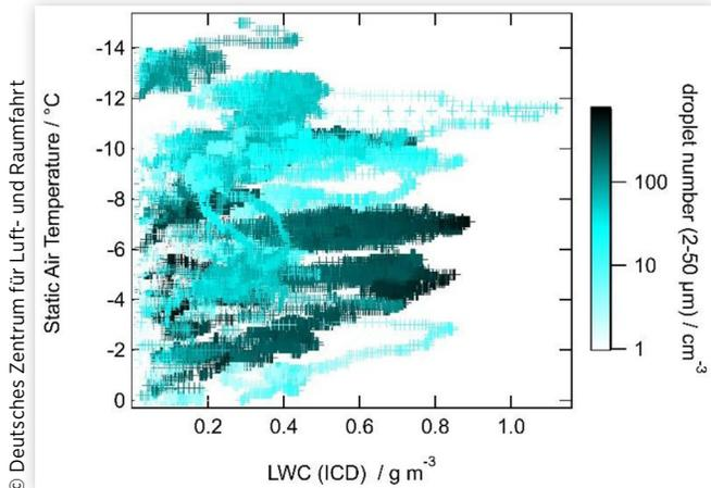
**FIGURE 13** Altitude profile of the LWC from flight on 23 February 2023 with SLD encounters. Large droplets with many small droplets have been reported in the two inversion layers at 800 and 1500 m.
