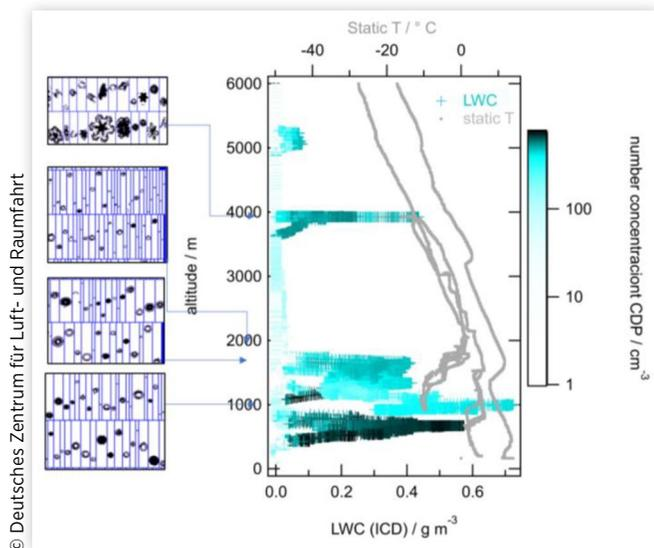
In the lower layer, several hundreds of small droplets were also measured indicated by the number concentrations of the CDP (color coding). At 4000m and temperatures of -15°C a mixed phase layer with larger ice crystals and large droplets was encountered. The lower layers in particular exceed the LWC range of the Appendix O envelope, which is reduced to values within the envelope if averaged over 30 s. Thus, relevant icing conditions as described Appendix O have been encountered on that day.
