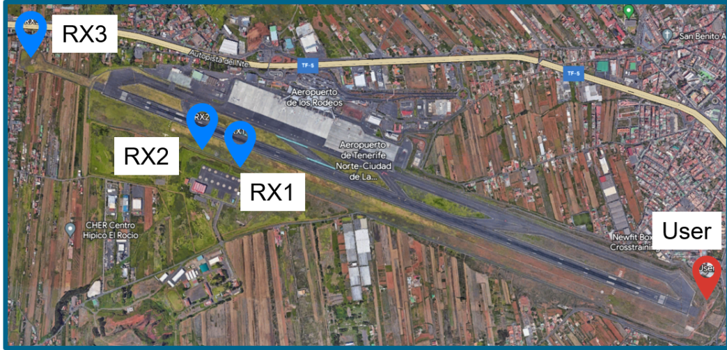
Figure 1: Experimental setup installed at Tenerife Norte Airport. The blue markers represent the location of three ground reference antennas, and the red marker the location of the ground user receiver.
