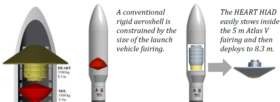
Figure 1: Rigid heatshield (MSL) and inflatable heatshield concept (HEART, NASA)
