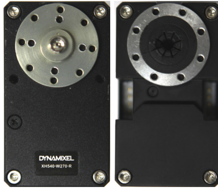
Figure 2.4: Photo of the front ( left ) and back ( right ) of a XH540-W270 servo. Note the hollow bearing, which allows routing cables through the joint axis.
