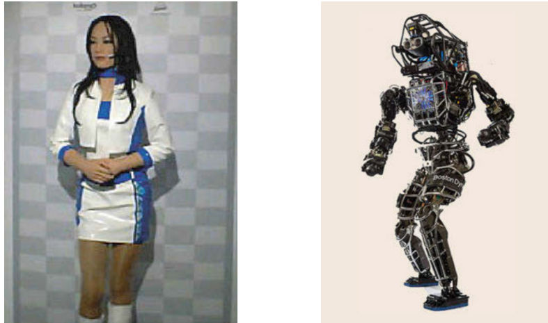
Figure 2.1: Comparison of the Actroid android robot ( left ) and the Atlas humanoid robot ( right ). [SK16, pp.1791-1792]
