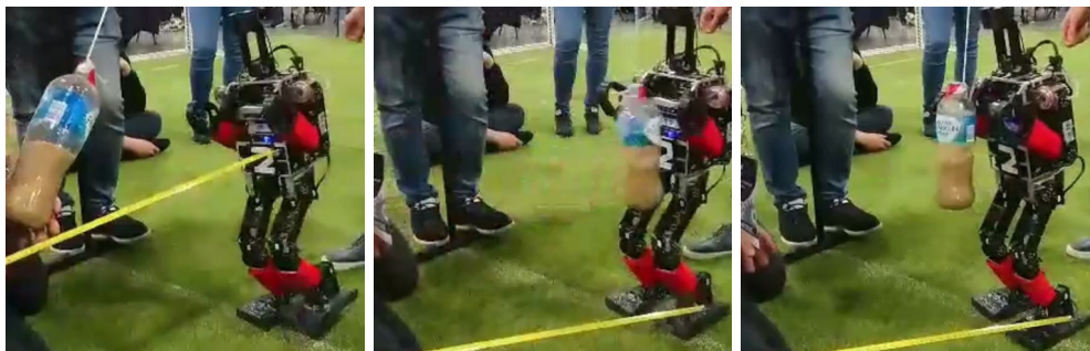
Figure 5.16: Images from the RoboCup push-recovery challenge. In the first image, the deflection of the weight (a bottle filled with sand) is measured, as this is the basis of the points that can be achieved. In the second image, the robot is hit by the weight. In the third image, the robot stopped walking and stabilized itself. See [1] for the video.
