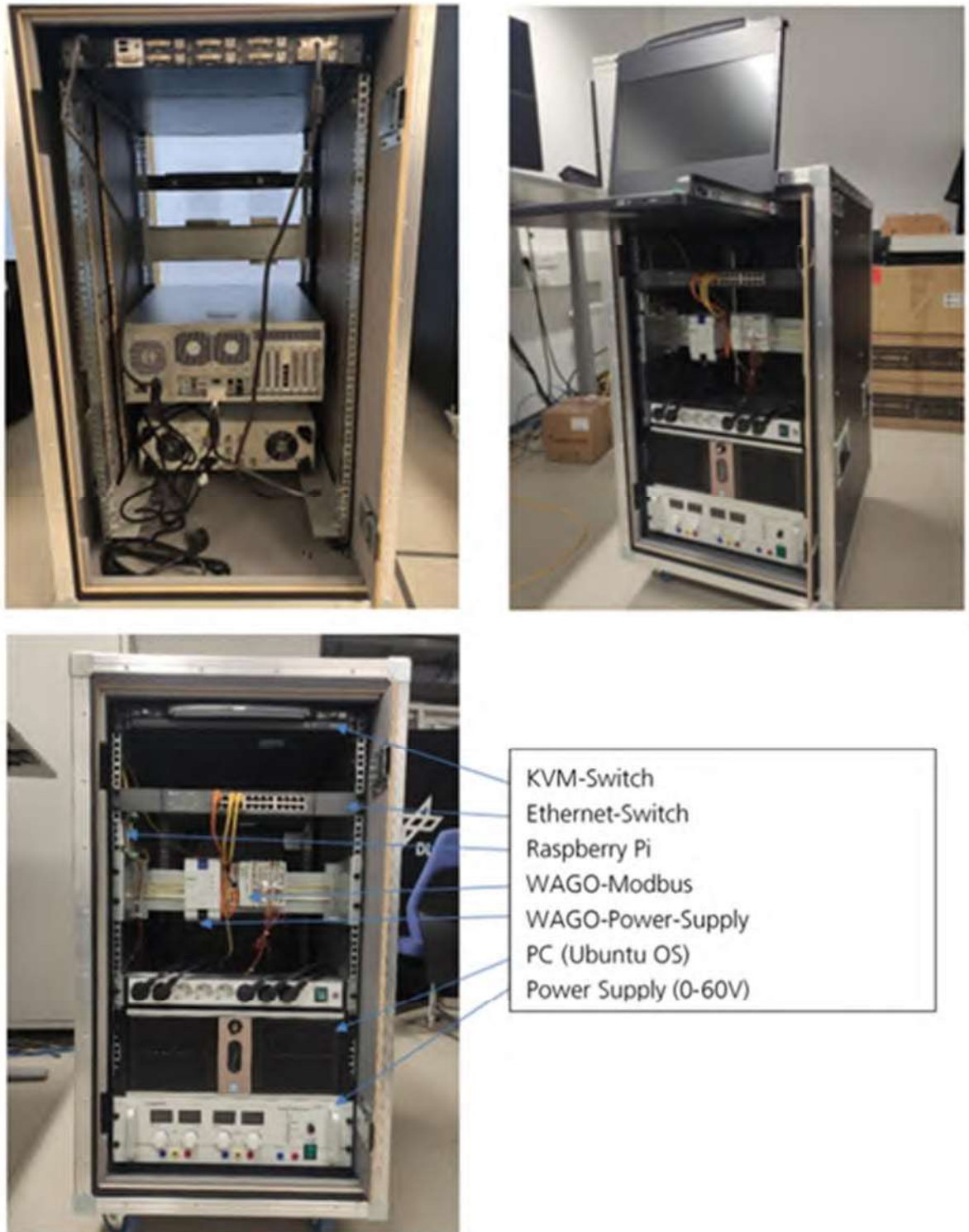
Figure 7-2: The mobile EULYNX Test Bench (Photos: DLR)
