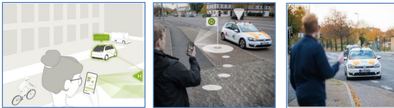
Fig. 6. DRT end user using prototype AR App for the localization of the virtual stop at the drop up location (DLR).
