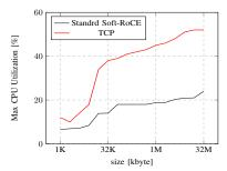
Fig. 6: Maximum CPU utilization with Soft-RoCE and TCP.
