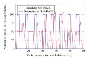
Fig. 12: Packets delivered in order with Deterministic Soft-RoCE and out of order with Standard Soft-RoCE.
