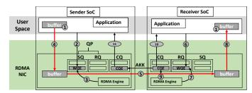
Fig. 4: Different components in an RDMA connection.
