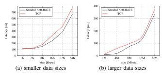
Fig. 5: Soft-RoCE vs TCP in terms of communication latency. is used by the network layer to route RoCE\_v2 data packets, which is similar to IPv6 addressing.
