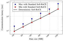
Fig. 13: Latency for a high-priority data packet.
