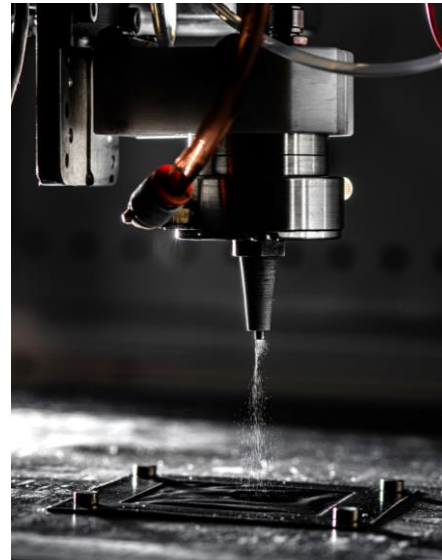
Ultrasonic spray coating
