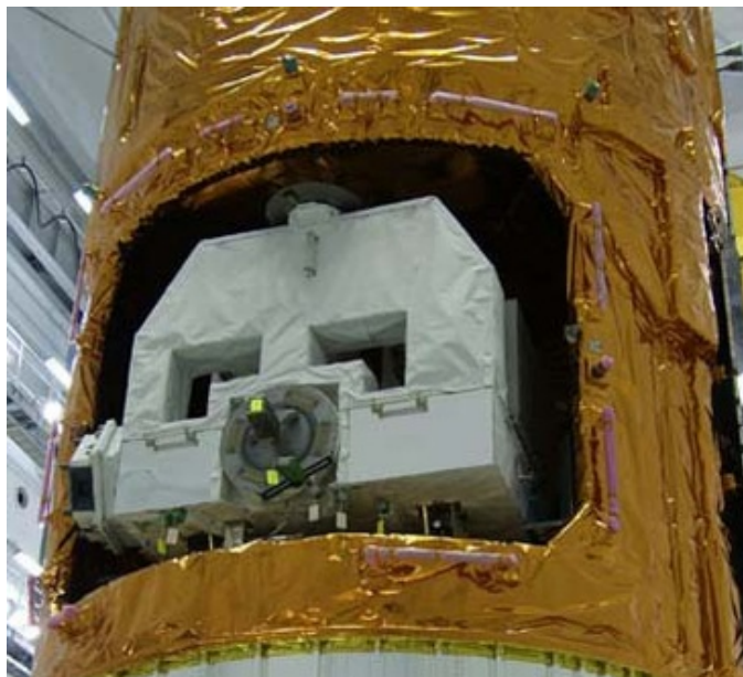
Figure 2.7: Exposed pallet inside the unpressurized logistics carrier of the HTV carrier. Image adapted from [33].
