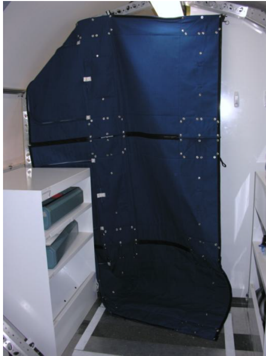
Figure 4.2: A privacy partition out of multipurpose cargo transfer bags (MCTB) used inside the habitat demonstration unit (HDU) for testing. Image adapted from [69].
