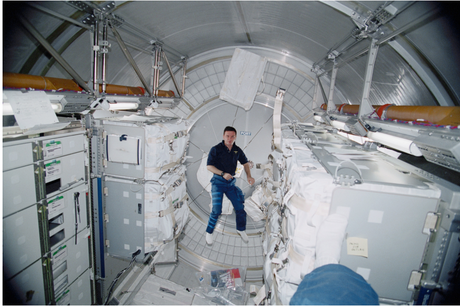
Figure 2.9: Interior of the MPLM Leonardo. Image adapted from [41].
