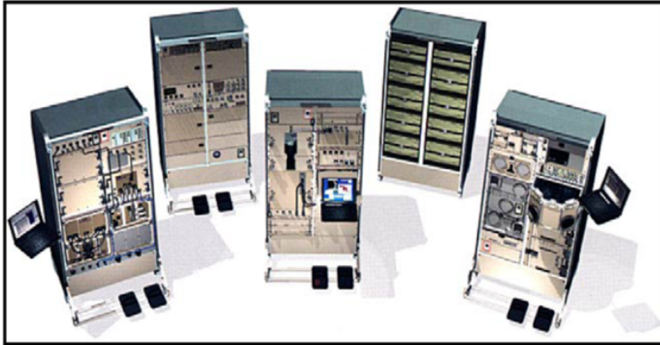
Figure 2.11: Five payload racks inside the Columbus laboratory on board the ISS. Image adapted from [45].
