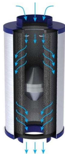
Figure 5-15 Example of an active air inline carbon filter [124]
