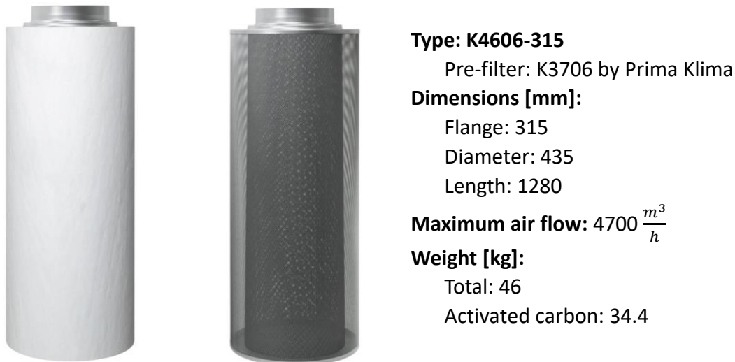
Figure 5-14 Carbon filter outside and inside view [123]
