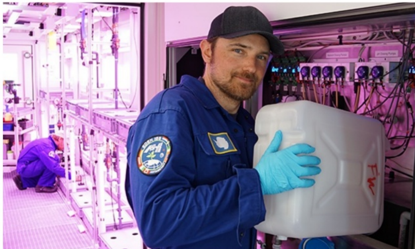
Filling the nutrient mixing tanks with water
