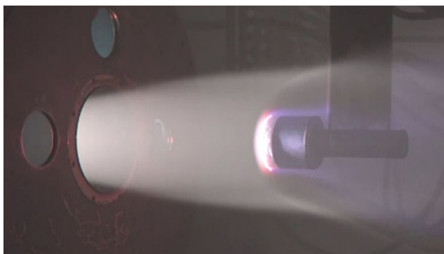
Figure 3. Representative photograph of an aerogel composite specimen (mullite composition) entering the arc-heated facility.
