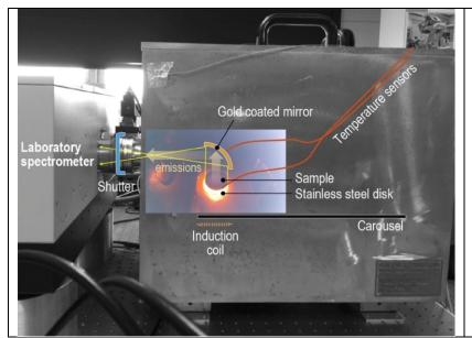
Side schematic view of the emissivity chamber at PSL
