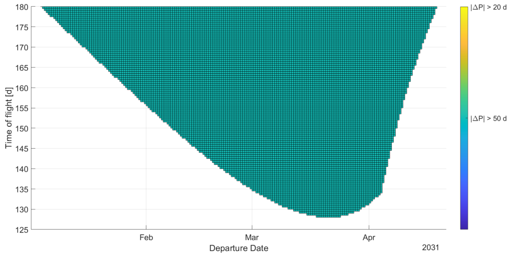
Figure 27: Porkchop plot displaying the values of \Delta P from equation (14). Indicates the possibilities of performing a free-return trajectory for all possible Earth-Mars trajectories in the 2031 launch opportunity.
