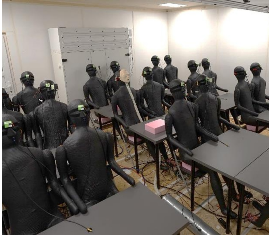
Fig. 8. Installation of the aerosol source on position I at seat D2.
