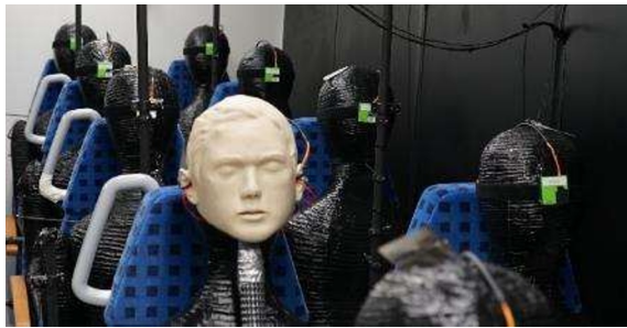
Fig. 4. Aerosol-exhaling thermal passenger manikin and particle concentration sensors in the breathing zones of all other passengers.
