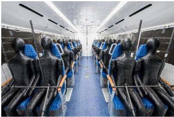
Fig. 1. View in the generic train laboratory fully equipped with thermal manikins.
