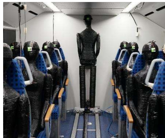
Fig. 3. Image of the walking thermal manikin in the generic train compartment.
