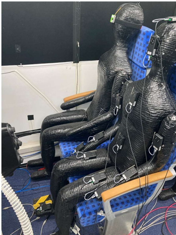
Fig. 3. Individual climate control system installed on the seat of the person in front with direction of influence on a thermal human model with 16 equivalent temperature comfort sensors.
