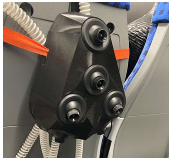
Fig. 2. Image of the personal multi-jet air nozzle.
