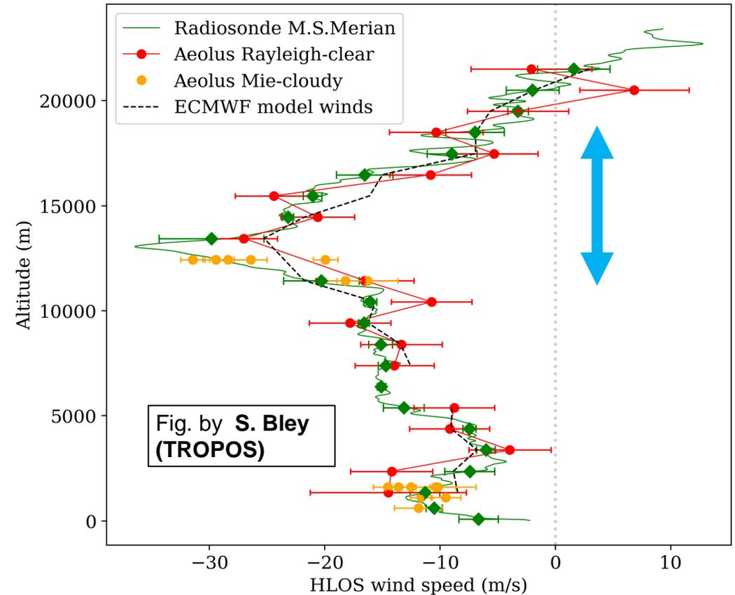
Fig.: Aeolus Rayleigh clear (red) and Mie cloudy (yellow) winds versus radiosonde winds (green) and ECMWF HLOS reference winds at Aeolus observation scale (dashed).
