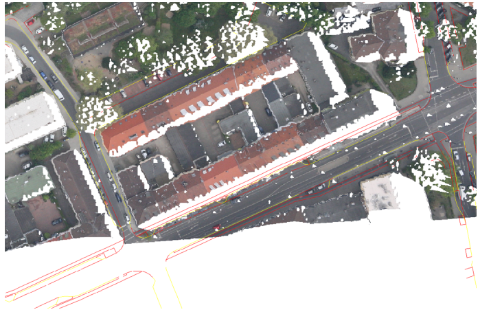
Fig. 5. Example of the curbstone polygons overlaid on generated ortho image. Occlusions due to sensor perspective lead to pixels with white color. Reference data in that area are to be excluded from the training procedure.
