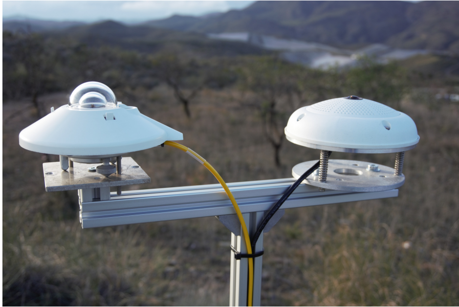
Figure 2.20: Illustration of the exemplary set-up of the PyranoCam method, consisting of an all-sky-imager in combination with a secondary standard thermopile pyranometer in a photovoltaic power plant, Photo @ Niklas Blum
