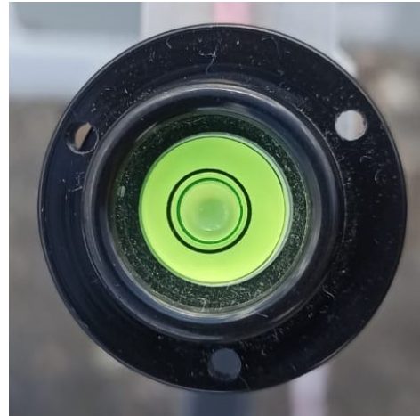
(b) Checking the leveling of the LI-COR 200R with the bubble level in position 180^\circ
