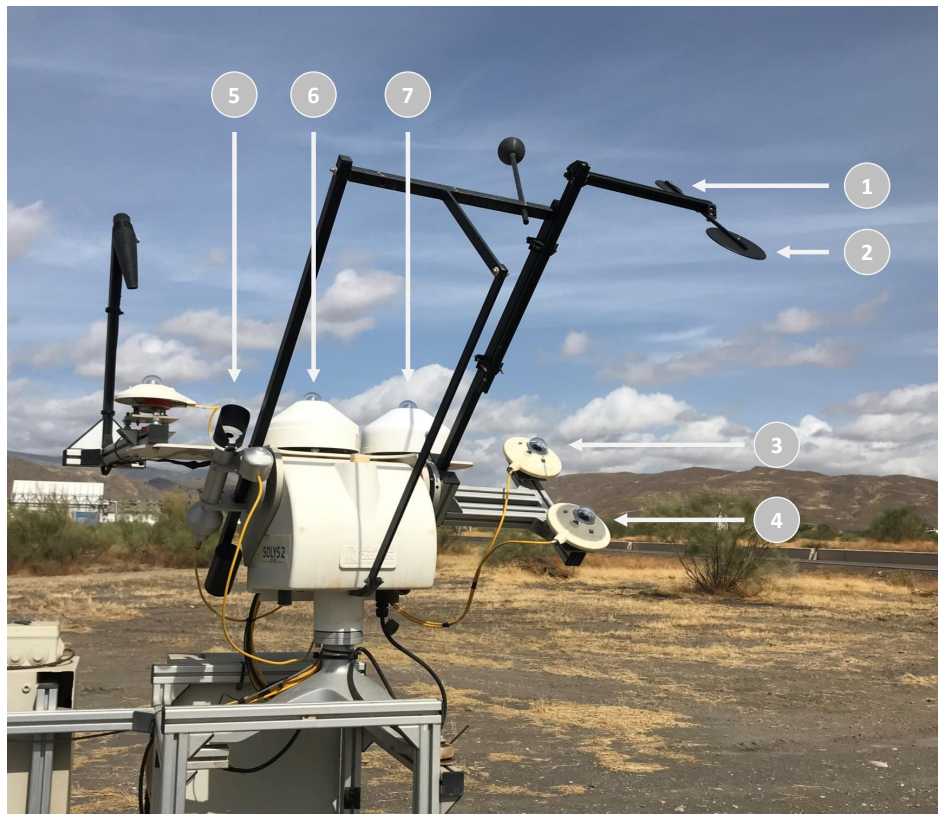
Figure 3.2: Used Sun tracker at the test site at CIEMAT's PSA, extended by the circumsolar irradiance measurement setup in the positions (1) to (4): (1) Small shade, (2) Wide shade, (3) pyranometer with an opening angle of \approx 2.5^\circ , (4) Pyranometer with an opening angle of \approx 5^\circ , (5) Pyrheliometer for reference DNI, (6) Pyranometer for reference GHI (moved on the tracker on 05/10/2022), (7) Pyranometer for reference DHI.
