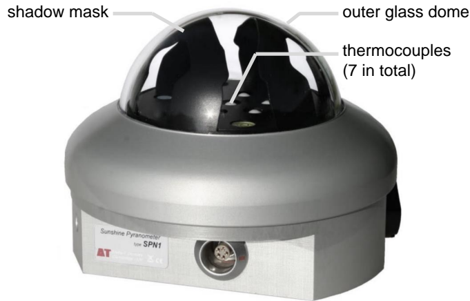
Figure 2.13: General technical design of Delta-T Devices' SPN1. Image taken from [32, p.3]
