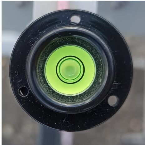
(a) Checking the leveling of the LI-COR 200R with the bubble level in position 0^\circ
