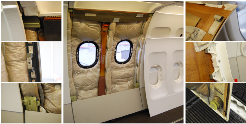
Figure 4.37: Typical joints of the inner side panel of an Airbus A320 11 with the finally fitted material parameters
