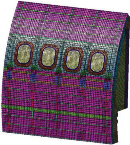
Figure 3.2: Detailed FE model of a realistic fuselage section including the outer skin, the insulation and inner side-wall panels (Source: [51, p. 6106]) 7
