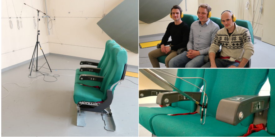
Figure 4.41: Experimental setup for characterisation of aircraft seats within the non-rectangular reverberation chamber at PTB Braunschweig; (a) Empty seats in central position, (b) seats with three passengers 14 and (c) intensity probe above the sitting surface
