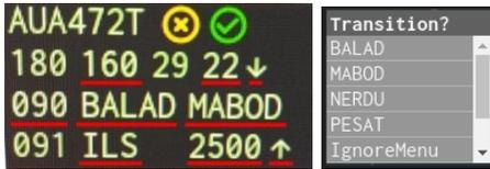
Figure 1. Left: Interactive radar label cells (red underlined); Right: Drop-down menu to enter given transition name, which opens with a click on the *transition* field (in this example the value *MABOD*). Yellow cross for rejecting all and green checkmark to accept all recognized values in the label.
