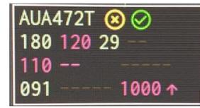
Figure 7. Radar label showing recognized flight level (120), heading (110 and “—” for waypoint (WP) cell), and descent rate (1000 or greater).
