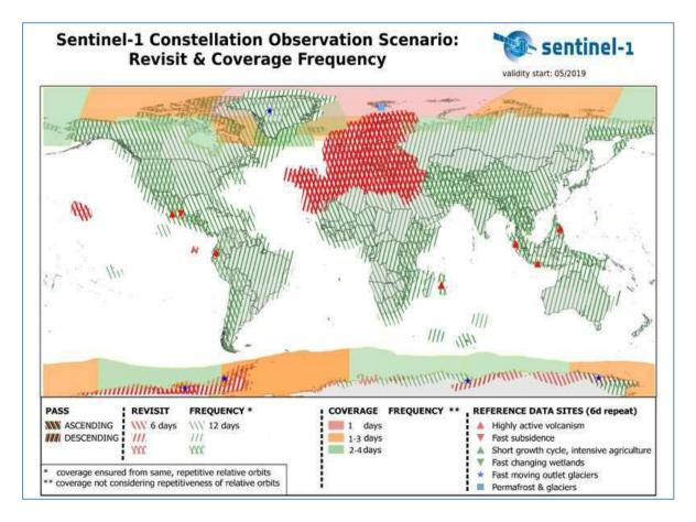
Figure 19. Illustration of the Sentinel-1 satellites revisit and coverage frequency.
