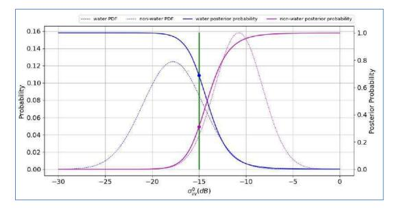
Figure 4. Illustration of the classification method used by TU Wien's flood mapping algorithm, based on the water and non-water probability density functions (PDFs), and water and non-water posterior probabilities with equal priors (0.5), for a flooded pixel.
