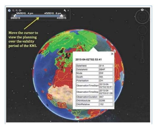
Figure 20. Illustration of the Sentinel-1 satellites schedule.
