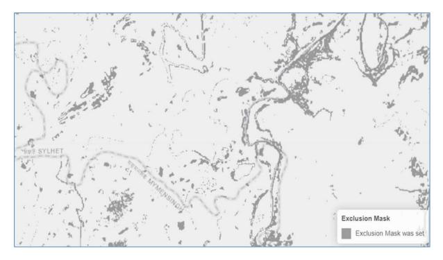
Figure 9: Example of the GFM Product output layer "Exclusion mask"
