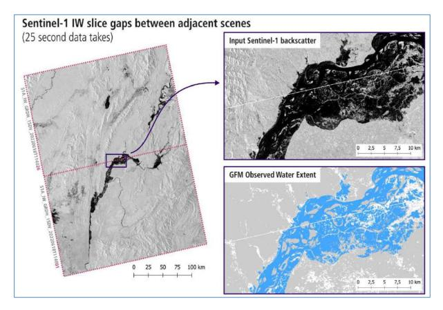
Figure 17. Example of linear gaps between Sentinel-1 acquisitions in GFM Product results.
