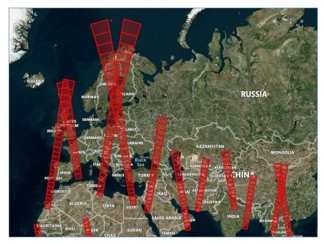
Figure 13. Example of the GFM Product output layer "Sentinel-1 Footprint and Metadata", showing incoming Sentinel-1 overpasses.
