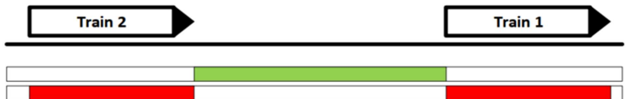
Figure 2: One train following another in Moving Block, from [1]. Green indicating the Reserved Area for Train 2, Red indicating the Occupied Track Status Areas
